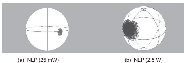
Fig. 9 Measured output polarization areas of NLP when the average power was changed.
